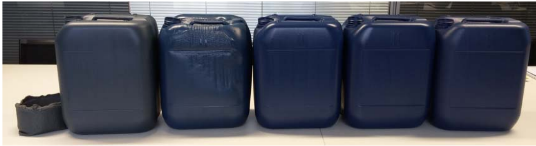
Jerrycans from different types of PE waste. Left: from traditional recycled PE; Right: from EXTRUCLEAN recycled PE
